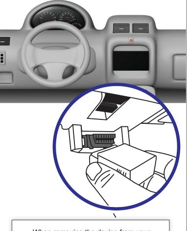
When removing the device from your vehicle, make sure you grasp the device as close to the port as possible. 2
